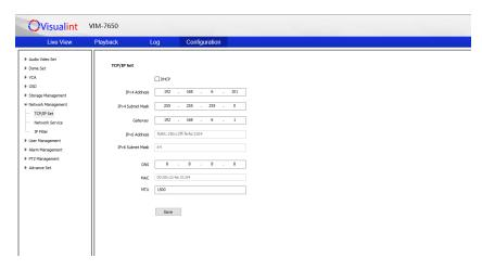
You can either enable DHCP with the checkbox, or manually enter an IP address and click Save. If you do, the camera restarts automatically.
